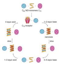
Buckybinding: The selective binding of either  $C_{60}$  and  $C_{70}$  in a mixture of the two fullerenes occurs by proton-induced, reversible, and controllable morphological switching between receptors for different fullerenes (see picture). Using hydrogen bonding as the exchange reaction, the response of the naphthalenediimide (NDI) building blocks to the presence of fullerene guests depends on the concentration of protons as a third component.
