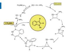
Dominos at zirconium: A cascade of N-N and C-H scissions and C-C and C-N coupling steps in the coordination sphere of zirconium directly converts alkynes and hydrazines into indoles. The reaction pathway differs fundamentally from that of the Fischer indole synthesis.
