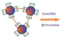
As few as 23 enzyme molecules could be detected on the basis of the dispersion of Au nanoparticles in a model bioassay whose sensitivity was boosted by the interplay between multivalent and monovalent supramolecular interactions: a
